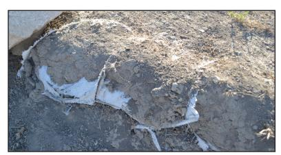
Figure 2: One of the synthetic bags split with the contents emptied, one year after installation (author's own image).
